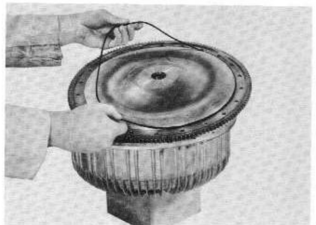
14. Install a new "o" ring gasket in the converter cover.
