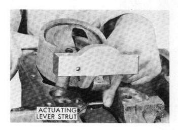
Position the servo actuating lever strut, and install the rear servo. Install the rear servo bolts, and torque them 40 to 45 foot-pounds.
