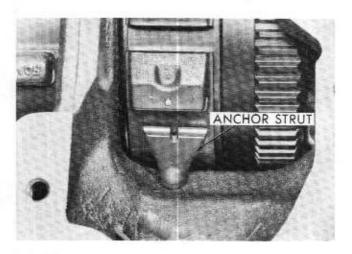
Place the servo anchor strut over the rear band adjusting screw head, which protrudes into the case, and rotate the rear band to engage the strut. Hold the strut in position.
