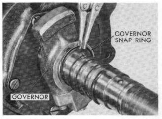
2. Install the governor -- indexing its groove with the ball, and install the governor snap ring.
