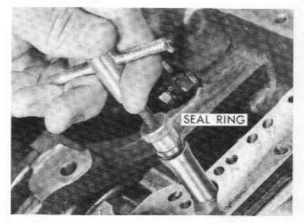
Install a new seal ring on the rear pump discharge pipe, and using a special tool, install the rear pump discharge tube in the case.
