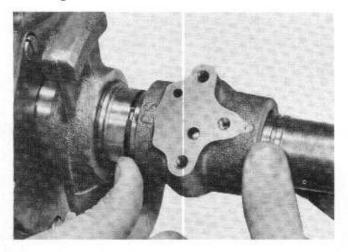
3. Install the distributor sleeve on the output shaft. Lubricate the parts to make installation easier.
