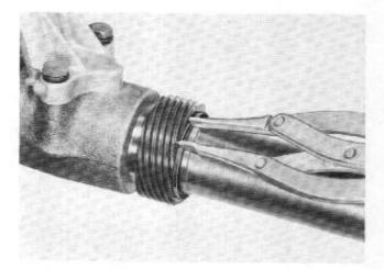
6. Install the speedometer drive gear, and the speedometer drive gear snap ring.
