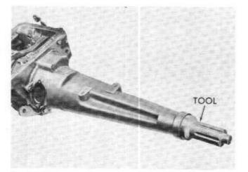
Using a rear extension housing seal installer, install the rear extension housing. Install the rear extension housing bolts and lockwashers...and torque 28 to 33 foot-pounds.
