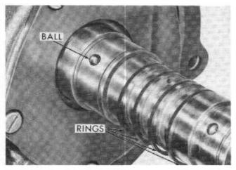
1. Install the governor drive ball in its pocket on the output shaft. Hold it in place with fluid.
