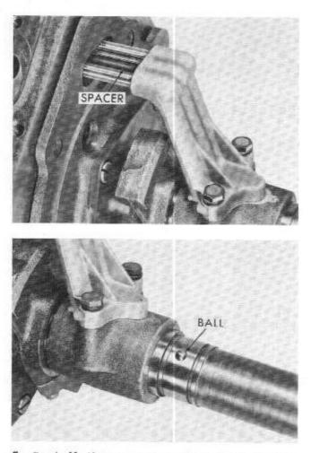
5. Install the speedometer drive gear ball in the output shaft. Hold it in place with fluid.
