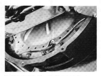
Remove the six flywheel-to-converter drive plate bolts.
