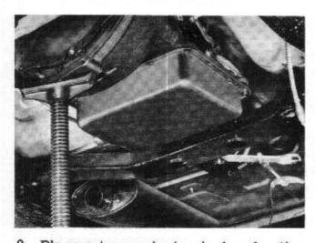
Place a transmission jack under the assembly, and raise it enough to take the weight off the cross member. Then, remove the cross member.
