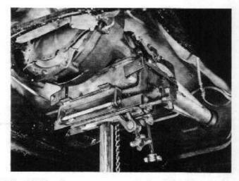
10. With the cross member removed, place a transmission-holding jack in position, and jack it up so that the transmission weight is fully supported by the jack.
