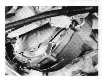
With a bracket, as shown, secure the converter in place.
