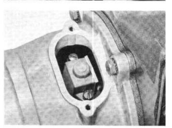
5. Remove the governor inspection cover, and apply air pressure to the front clutch passage in the case. Listen for a sharp click, and observe whether the governor valve snaps inward. If the valve moves inward, correct valve operation is indicated. If the valve doesn't move inward, repair or replace the governor.
