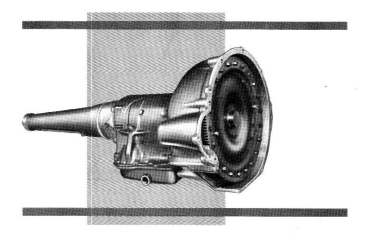
This manual covers a basic type of automatic transmission used in Ford Motor Company products. In Ford, it is called the Fordomatic; in Mercury, the Merc-O-Matic; in Lincoln, the Turbo-Drive.
