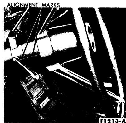
FIG. 17—Typical Straight-Ahead Position Marks
