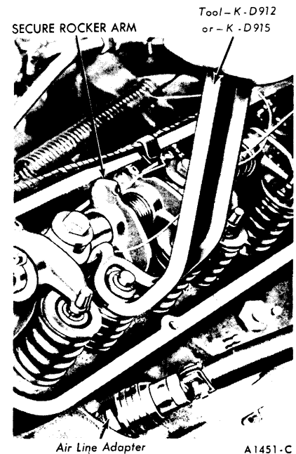
FIG. 26—Compressing Valve Spring—In Chassis
