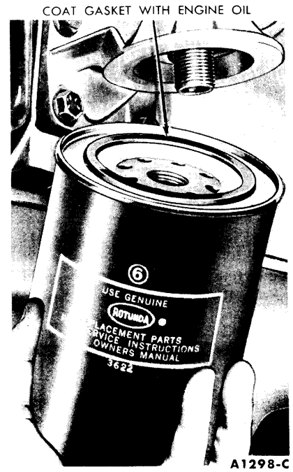
FIG. 48—Rotunda Oil Filter Replacement
