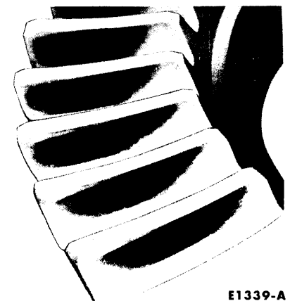
FIG. 5—Acceptable Non-Hunting Pattern—Center-Heel-Center
