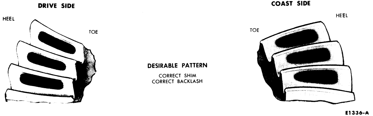
FIG. 2—The Ideal Tooth Pattern
