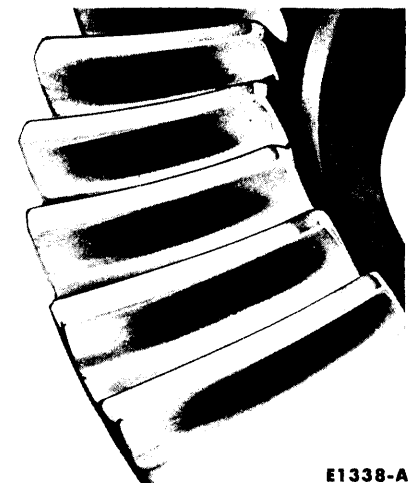
FIG. 4—Acceptable Non-Hunting Pattern—Center-Toe-Center
