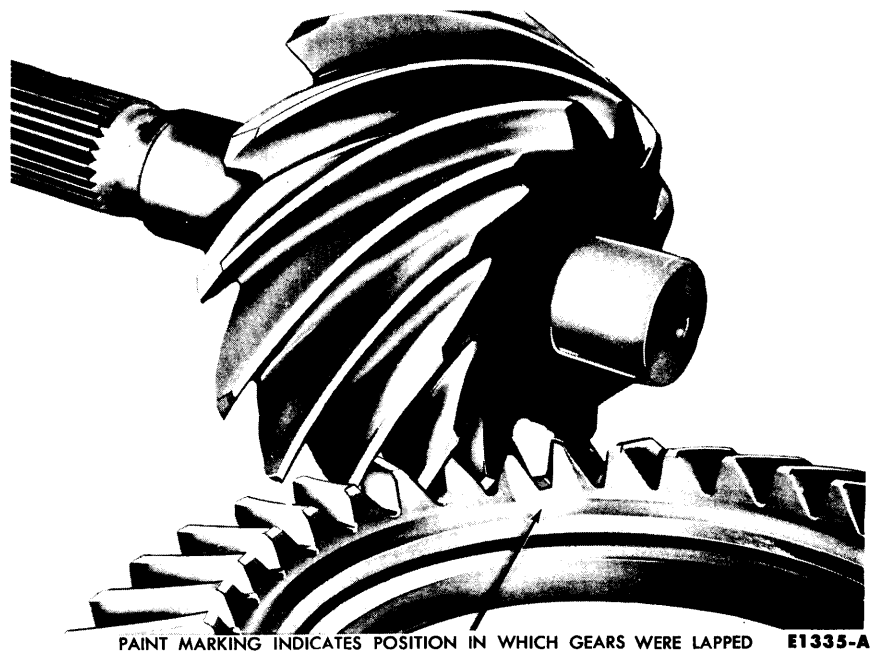
FIG. 35—Gear Set Timing Marks
