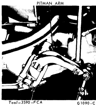
FIG. 12—Removing Pitman Arm
