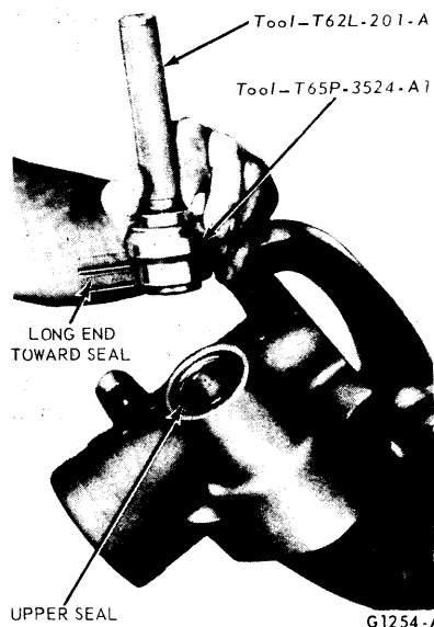
FIG. 30—Installing Sector Shaft Inner Seal
