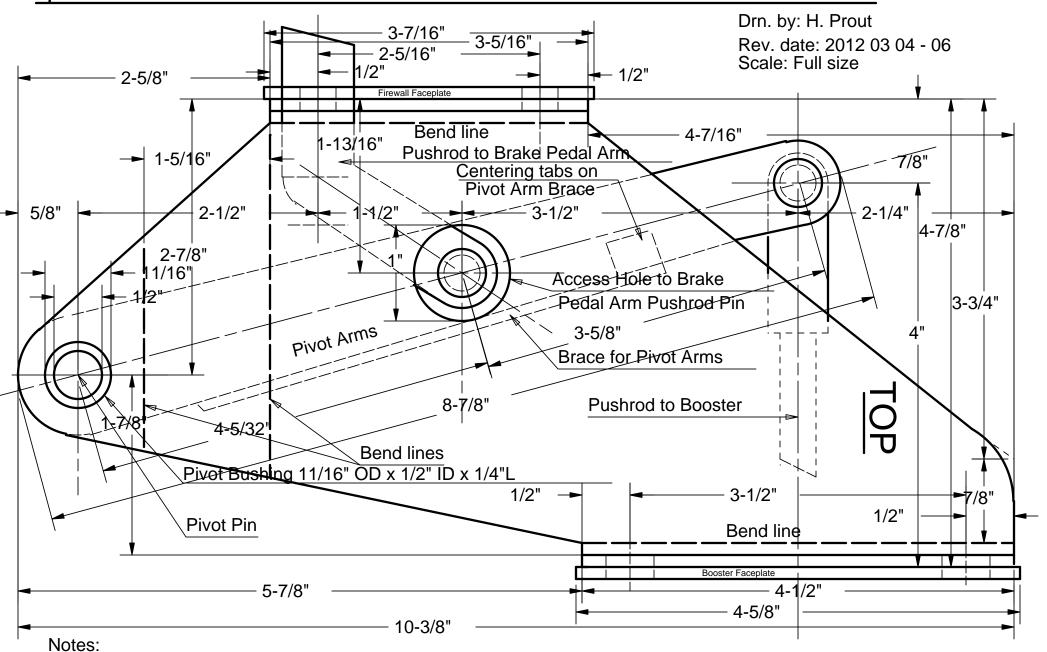
Two Bracket Pieces req'd. - one left and one right Weld pivot bushings to bracket plates
