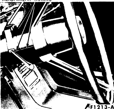
FIG. 1—Typical Straight Ahead Position Marks
