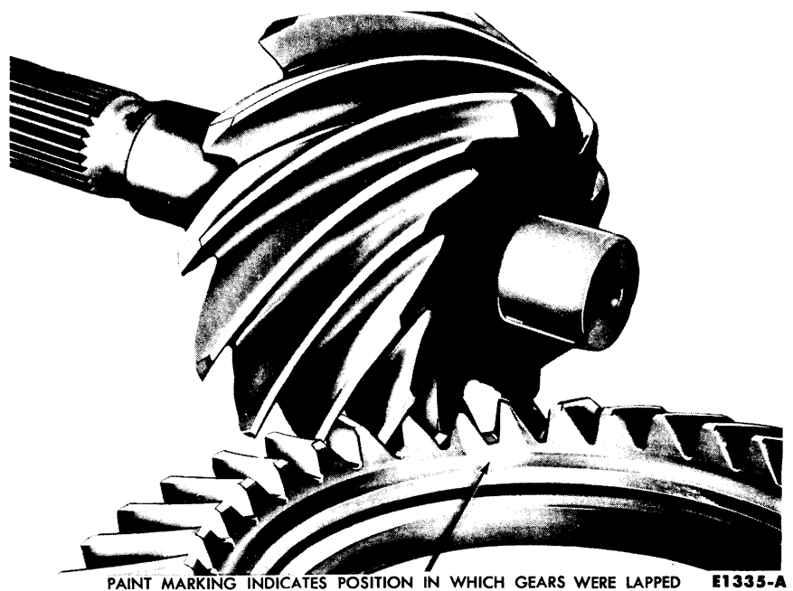
FIG. 35—Gear Set Timing Marks
