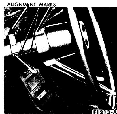
FIG. 17—Typical Straight-Ahead Position Marks
