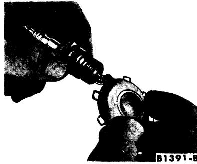
FIG. 4—Gapping Spark Plug
