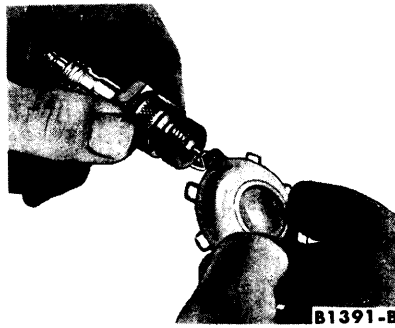
FIG. 27—Gapping Spark Plugs
