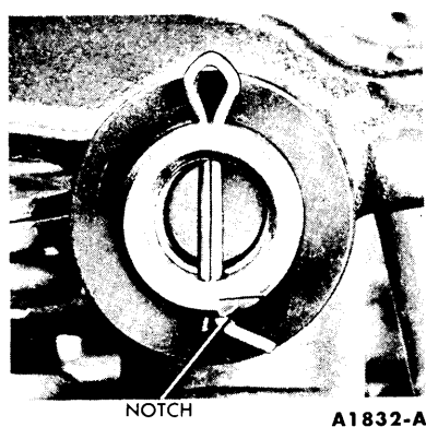
FIG. 15—Typical Installation Identification Mark—Rocker Arm Shaft Assembly
