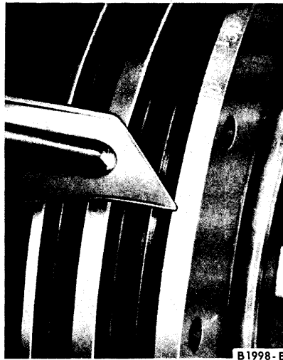
FIG. 25—Typical Timing Marks
