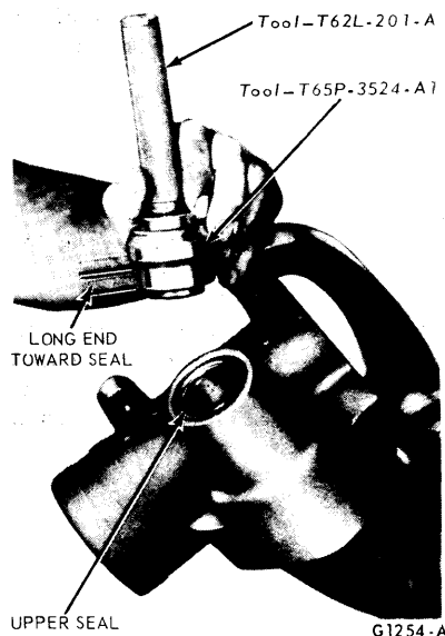
FIG. 30—Installing Sector Shaft Inner Seal
