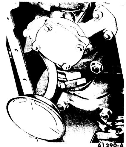
FIG. 49—Oil Pump and Inlet Tube Installed
