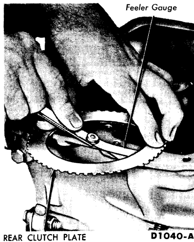
FIG. 19—Check Rear Clutch Steel Plate Coning
