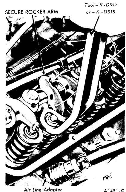
FIG. 26—Compressing Valve Spring—In Chassis
