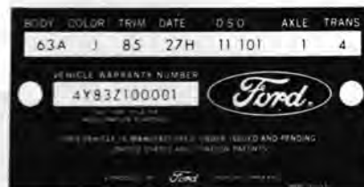
The Thunderbird patent plate is located on the left door lock face panel.
